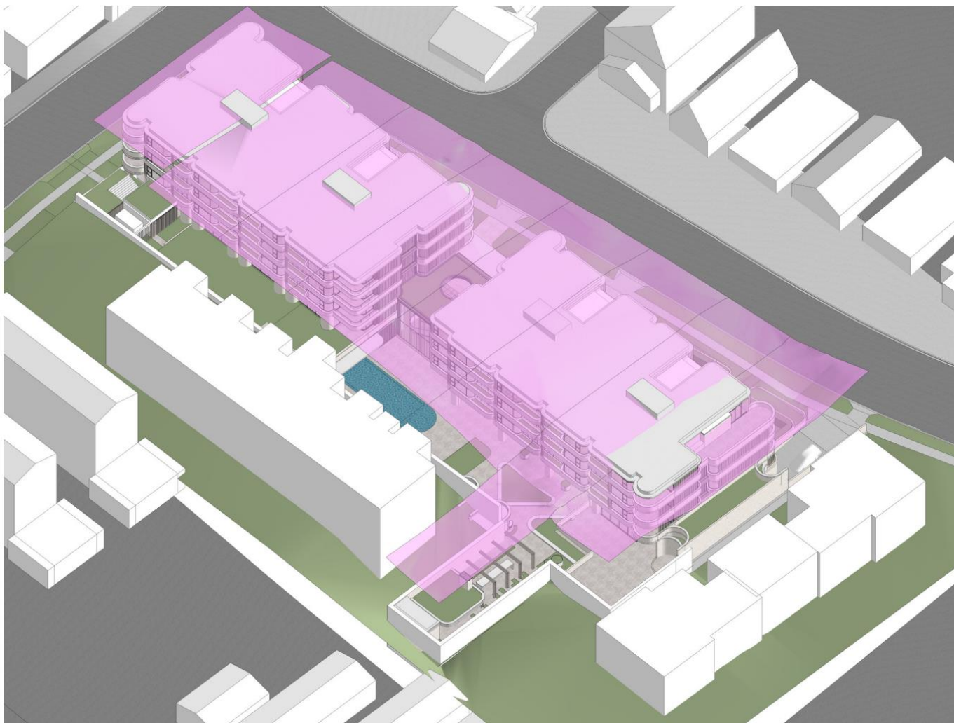
Figure 4: Extract of Building Height Plane (Page 13 of DA RFI Design Response prepared by Bates Smart) - non-compliant elements illustrated in grey.
